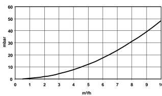
$m^3/h$  = Through put flow rate mbar = Through put resistance
